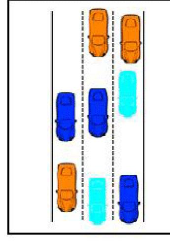
Level of Service E: Unstable flow at or near capacity levels with poor levels of comfort and convenience.
