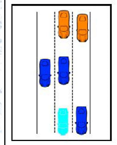
Level of Service D: High-density flow in which speed and freedom to maneuver are severely restricted and comfort and convenience have declined even though flow remains stable.
