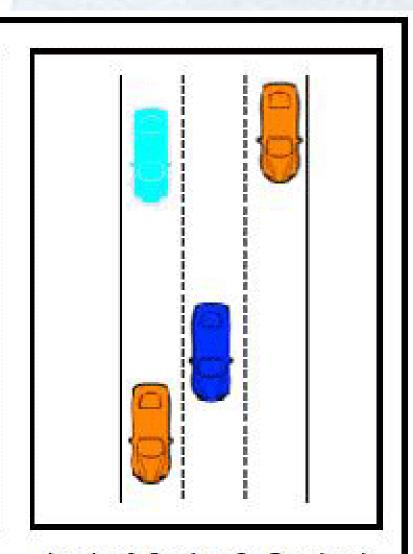
flow that remains stable but with significant interactions with others in the traffic stream. The general level of comfort and convenience declines noticeable at this level
