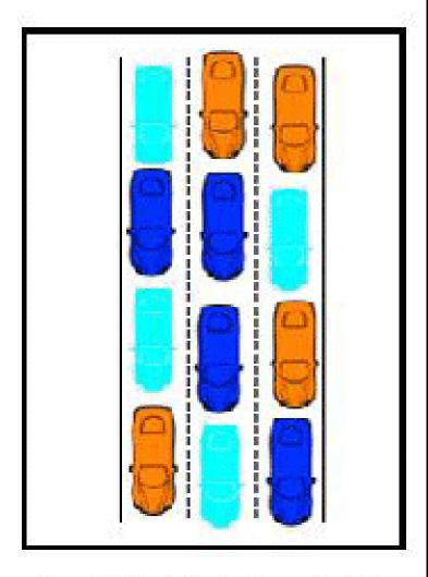
Level of Service F: Forced traffic in which the amount of traffic approaching a point exceeds the amount that can be served. LOS F is characterized by the stop-andgo waves, poor travel times, low comfort and convenience, and increased accident exposure.
