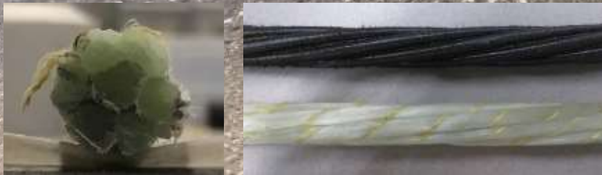
(a) GFRP strand prototype cross section; (b) compared to a CFRP alternative.
