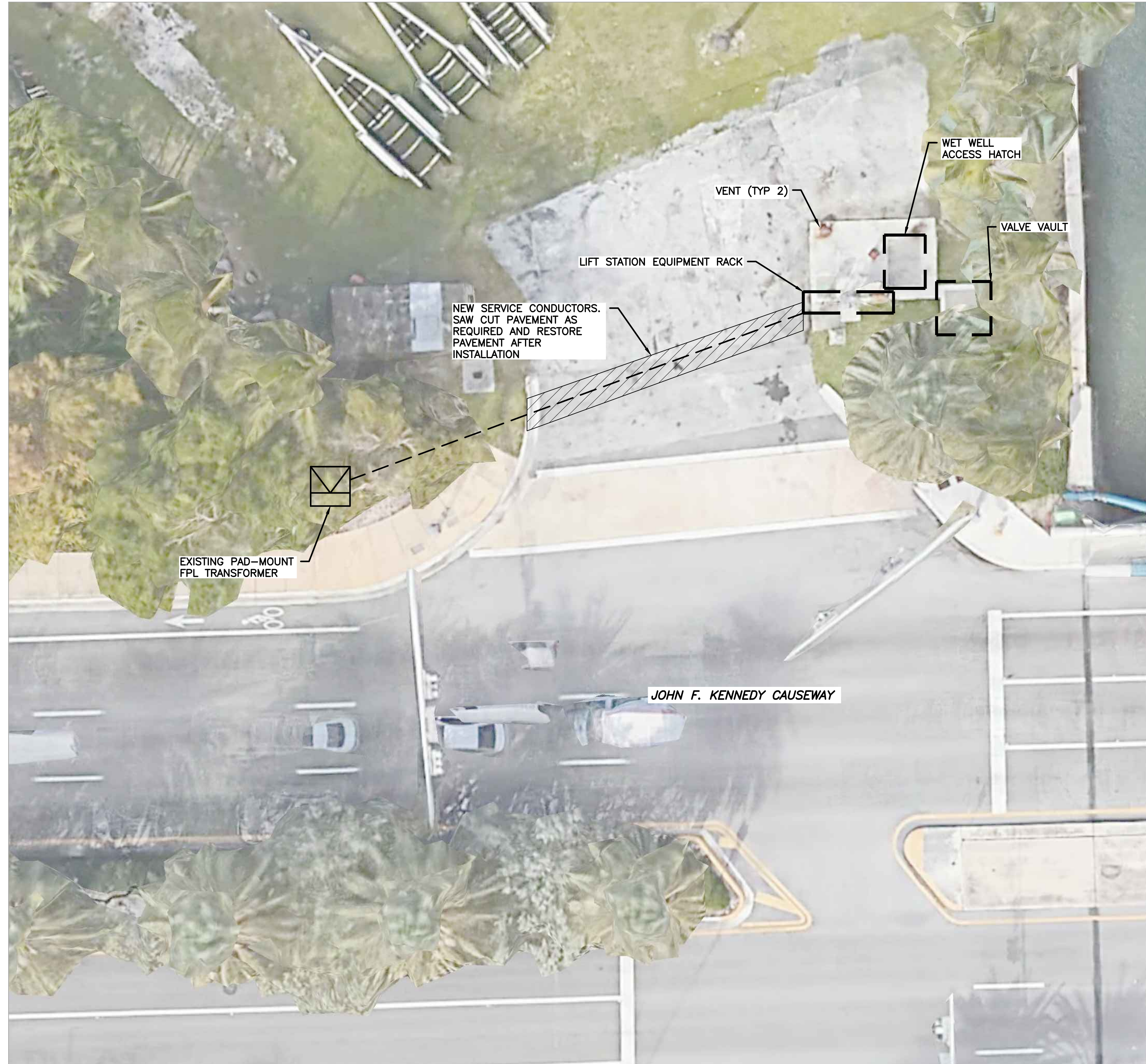
ELECTRICAL SITE PLAN SCALE: 1"=10'-0"
